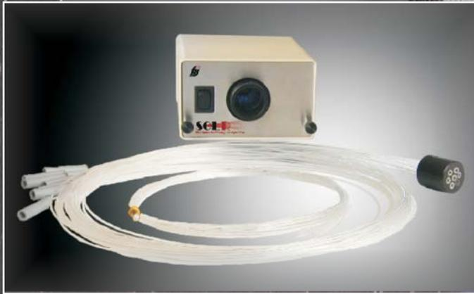
The StarScape system is comprised of three components: the light source, a SOL-R 3575 reconfigurable quartz halogen power supply which accepts 35, 50, or 75W 12 volt MR16 lamps, the preassembled and polished extension harness and various star bundles. 16 standard stocked parts can create star fields ranging in size from 100 to 1200 sq feet in area, with densities ranging from .5 to 5 stars per sq foot.
