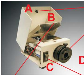
A Plastic pin secures cover and facilitates quick, easy lamp change.
